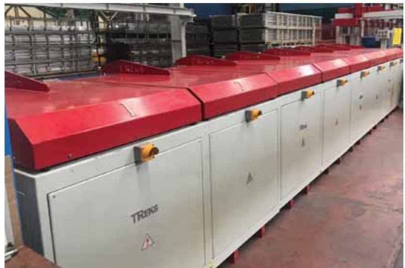
Smart die oven, thanks to its unique software prevents the over fast and over heating of the die and therefore offers long die life.
